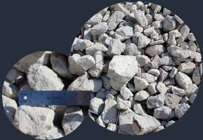
OVERSIZED CRUSHED CONCRETE
